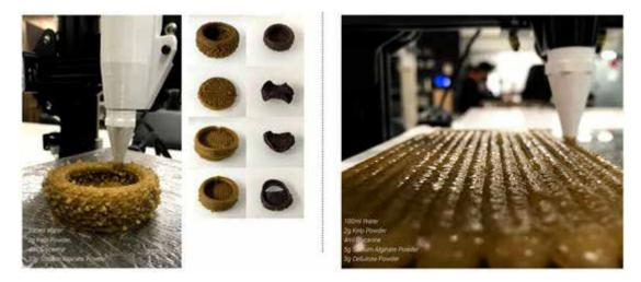
Figure 4: (top) Initial 3D Printing Extrusion Tests of Seaweed Biocomposite.
