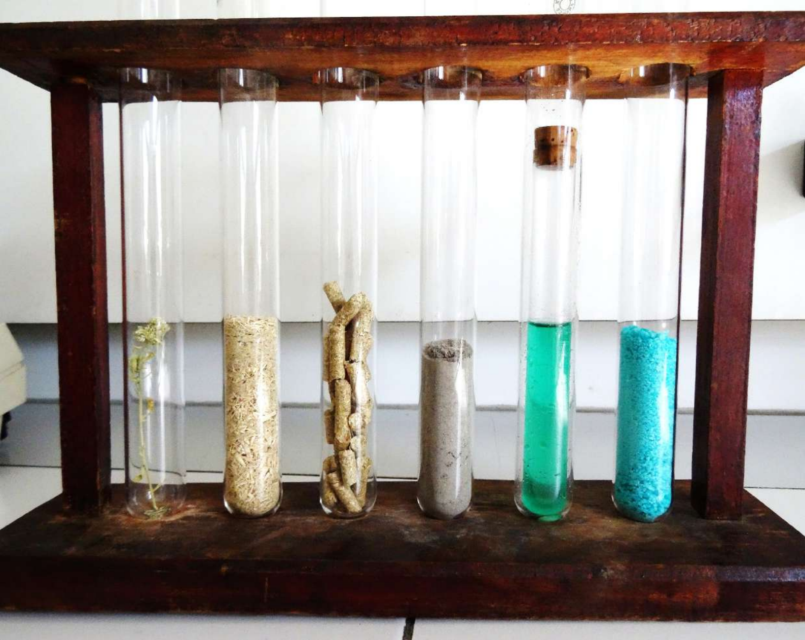
Figure 1: Steps from the hyperaccumulator plant (left-side tube) to one bio-sourced metallic product (here nickel sulphate on the right-side tube)
